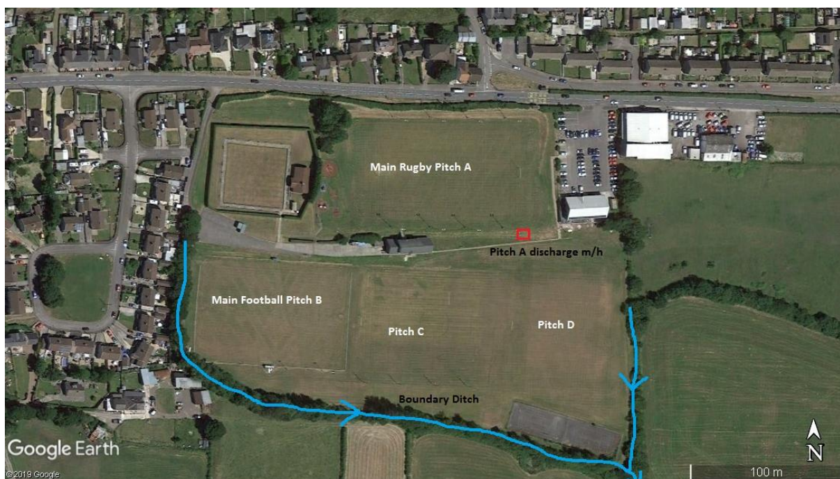
Figure 11 - Likely discharge point for pitch A, also shows the boundary ditch Other observations
